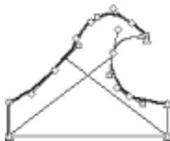
Figure 6: The repeating shape used to create the design in Figure 1 is shown with all points selected. The left and right sides of the base are designed as complementary so that a seamless transition is created when the shape is tiled.
